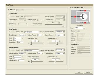
Figure 5. Easily configure an I-V characterization test with the Parametric Measurement Manager Pro software.
